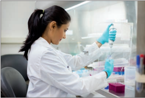
Figure 1.4. Experiments are one way that we obtain facts. This picture shows a scientist using a micropipette, an instrument designed to transfer tiny, precisely measured volumes of liquid.
