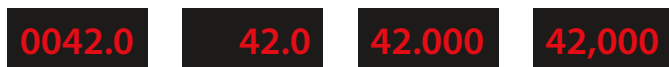
Figure 1.3. With digital instruments, all digits are significant except leading zeros. Thus, the numbers of significant digits in these readings are, from left to right, three, three, five, and five.
