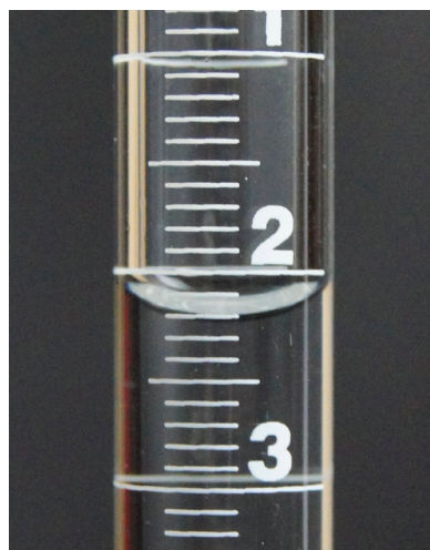
Figure 1.5. Reading the significant digits on a buret.
