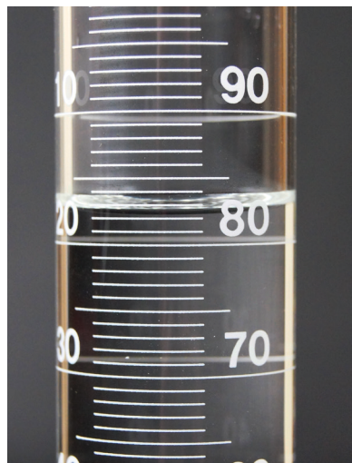
Figure 1.6. Reading the significant digits on a graduated cylinder.
